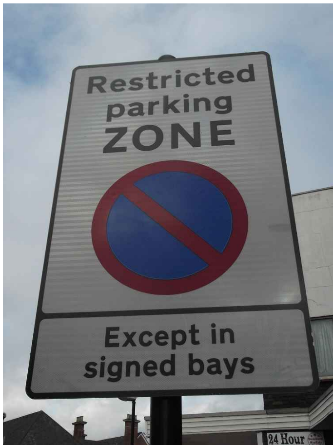
An entry sign to an RPZ. The circle means 'no waiting' and the sub plate excludes signed bays which could be for parking, loading, bus stops, taxi ranks and other bay types.
