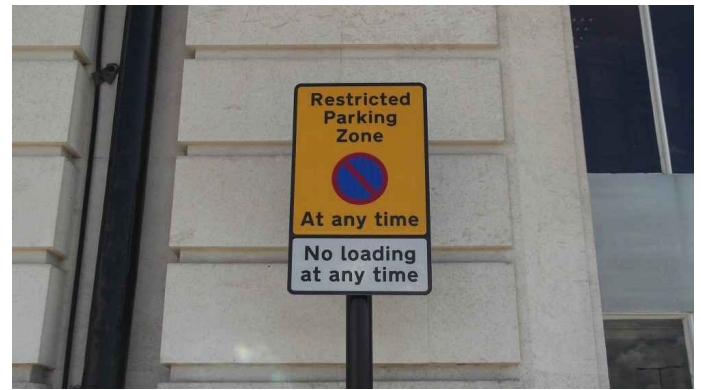
A repeater sign in an RPZ. The yellow sign replaces the need for waiting restrictions (double yellow lines in the case of 'at any time' controls) and the white sign replaces a loading ban (which would otherwise be pairs of yellow kerb blips).
