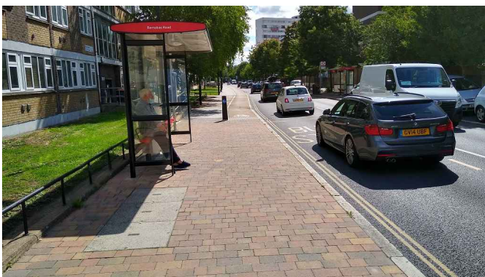
Space shared between people walking and cycling. This is less desirable, but in this example, at least the clutter has been kept to a minimum to maximise space.
