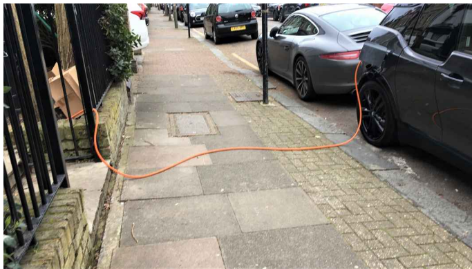
A private charging cable left across the footway which creates a trip risk.
