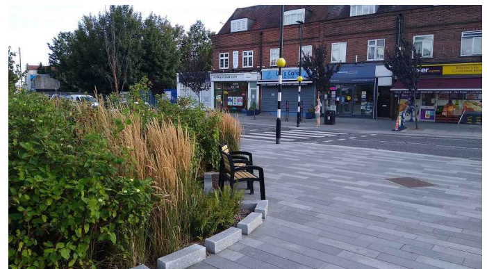
Seating recessed into a landscaped area reduces clutter on the crossing desire line.
