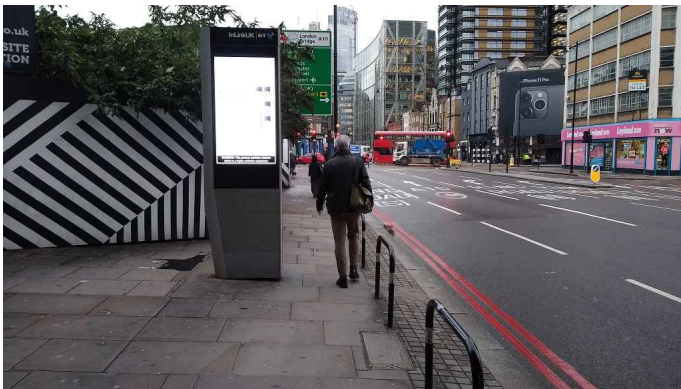
Electronic monolith which is restricting the effective footway width.
