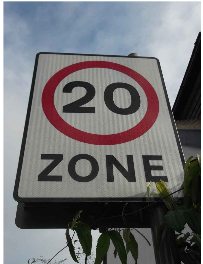
Speed limit signs are regulatory signs. 20mph Zones apply on an area basis.
