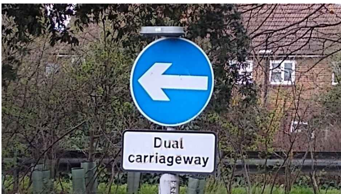
Regulatory turn left sign, the sub plate explains that drivers are entering a dual carriageway.
