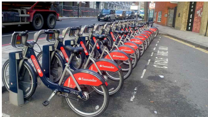
Hire cycle docking station within an on-carriageway bay.
